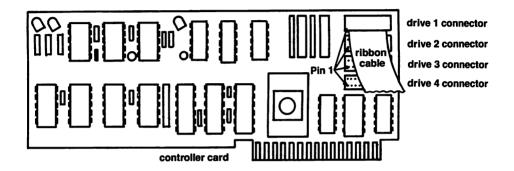
Fig. 1-1: Elite Controller Cable Connections
