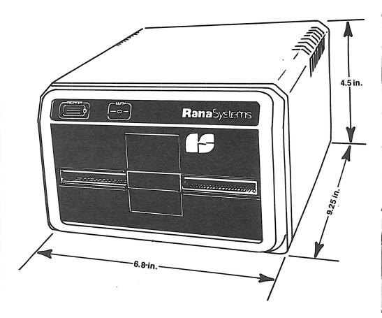
Fig. 6-8: Physical Dimensions of Elite Drives
