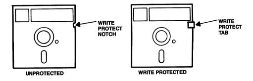
Fig. 8-1: Write Protecting Diskettes
