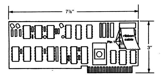
Fig. 6-9: Elite Controller Physical Dimensions
