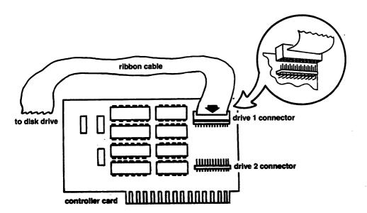
Fig. 1-2: Disk-II Controller Cable Connections
