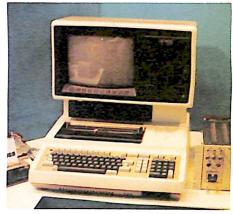
How about a keyboard, numeric pad, printer, two minifloppies and a CRT in one enclosure? This one is called the if 800.
